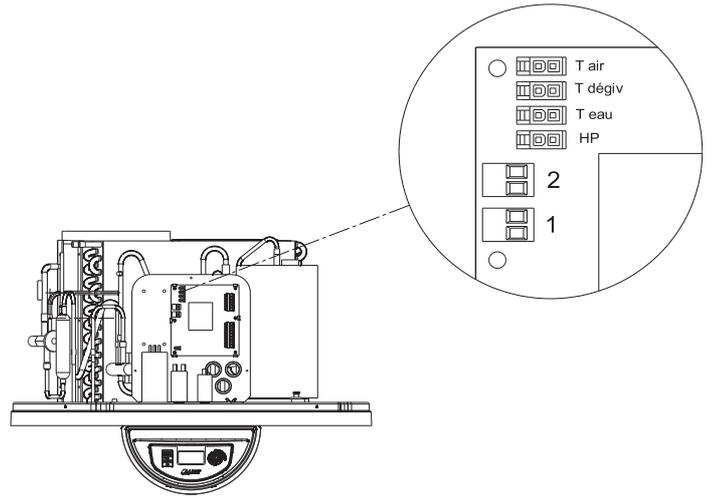
Only a zero-voltage, external control such as a timer switch should be used ( if not, the electronic board could be destroyed)
